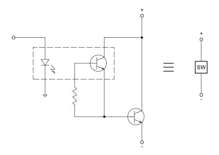
Figure 5.3 Isolated Loop Current Switch
